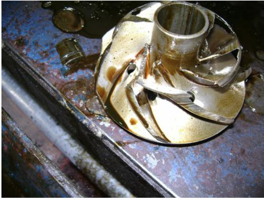
Figure 4.9 Pump stages wear
