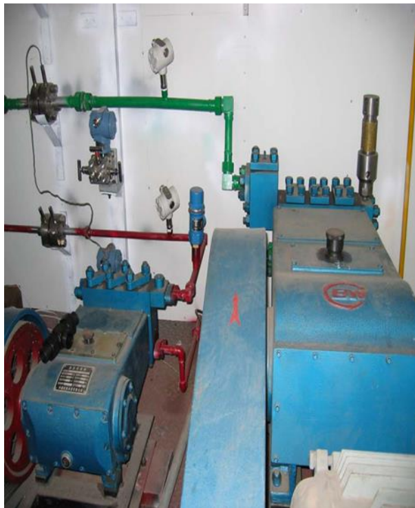
Figure 4-5 Controllable convert-frequency feed oil and feed water system
