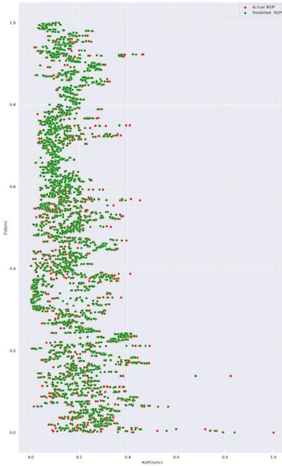
Figure 2.6 Actual and predicted ROP for the new well
