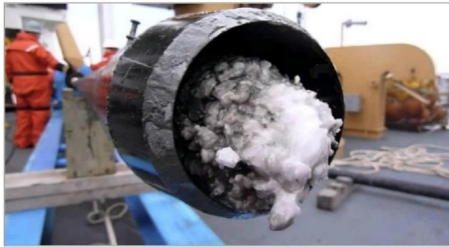
Figure (2.17) Gas hydrate plugging of gas transportation pipeline (Polartrec.com)
