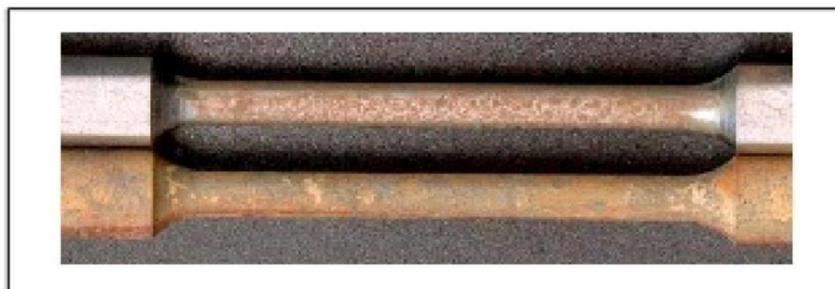
Figure (2.18) General view of corrosion damage of the specimen after exposure to gas hydrates (Poberezhny, et al 2019).
