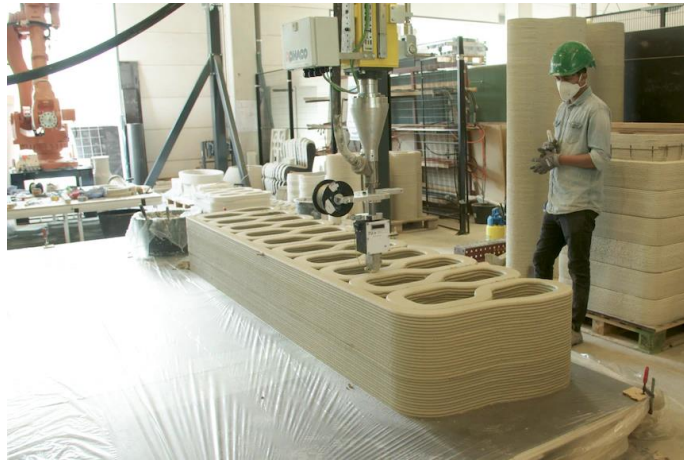
Figure 1-6 . 3D printing process of building parts [3].
