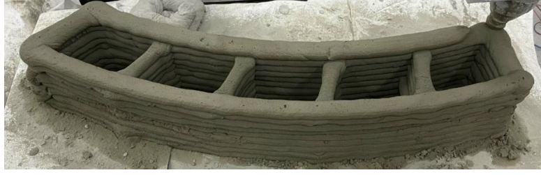
Figure 2-4 Realistic wall structure after concrete 3D printing.
