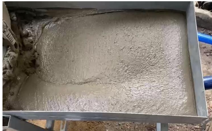
Figure 8-6 Concrete is turned continuously to avoid material stratification.
