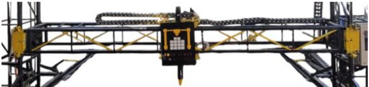
Figure 8-2 . X-axis horizontal beam and actual extrusion unit.
