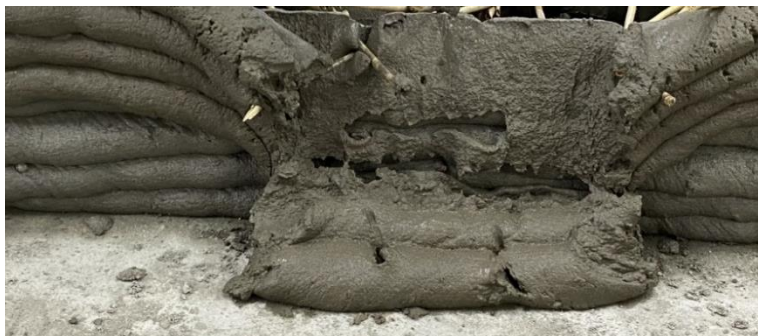
Figure 2-7 Structural failure is caused by a mixture of materials that does not achieve ductility.
