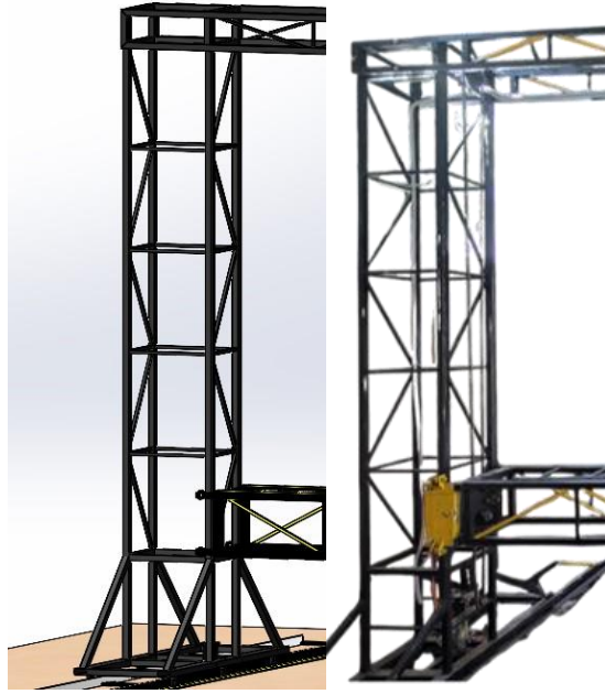
Figure 8-3 The body pillar assembly of the machine, (a) By design, (b) In fact.
