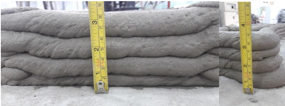
Figure 2-8 Deformation of the printing layer without gypsum powder.
