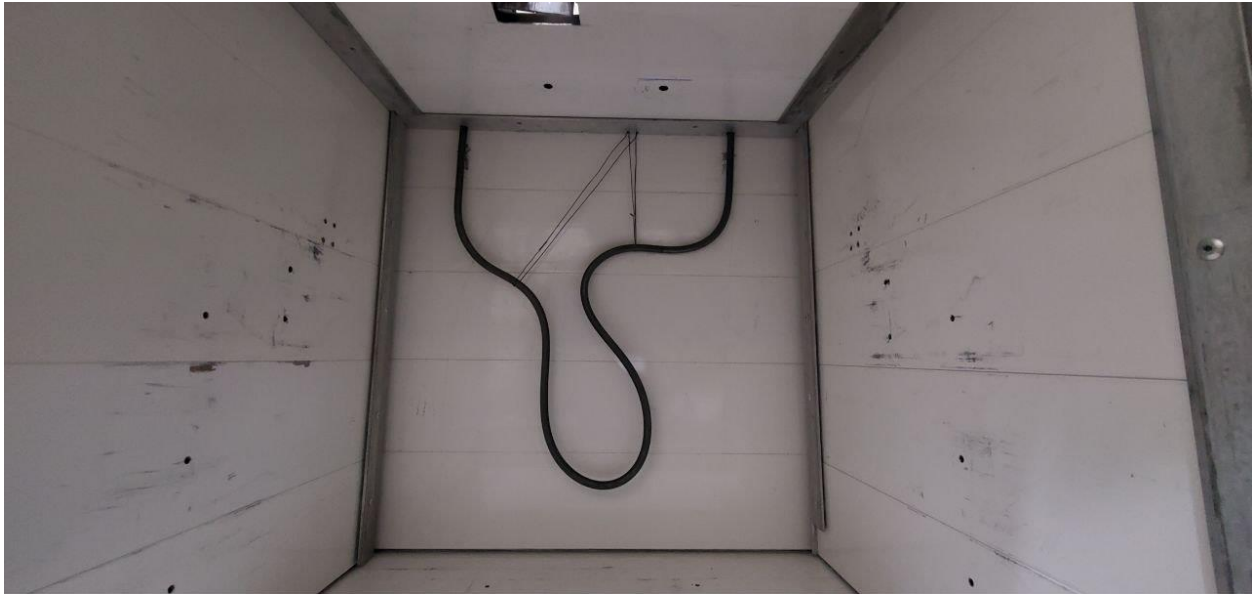
Figure 4.34 Thermal film installed inside the printer behind the insulation wall, one meter long, from the local market
