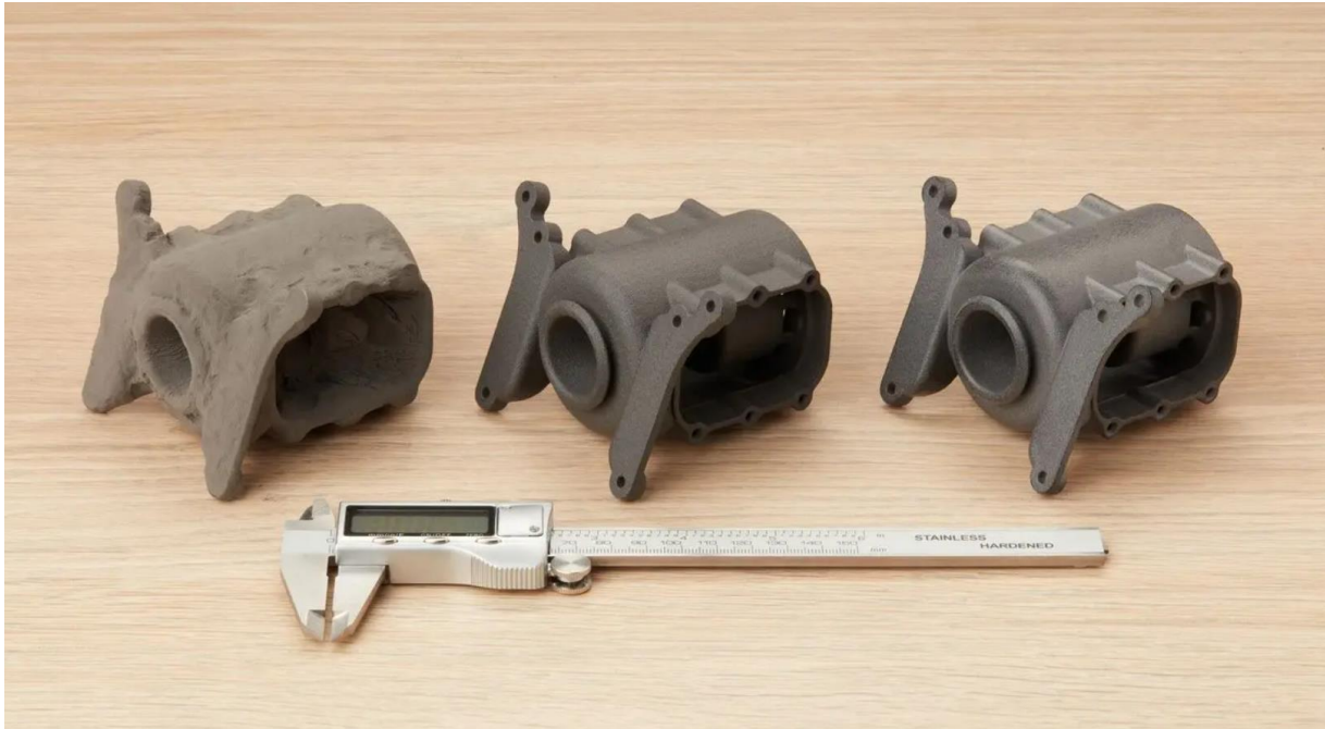
Figure 3.14 Example of what the part looks like before and after the final processing stage before use.
