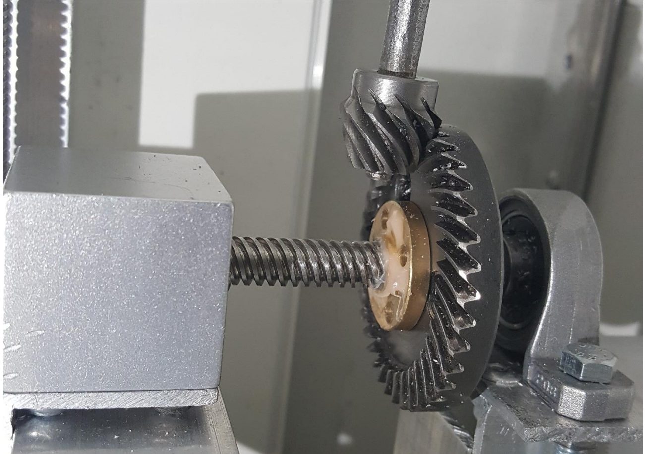
Figure 4.27 Converting the vertical movement on the Y axis to the horizontal movement on the Z axis in the scanner that transfers the powder to the printing medium.
