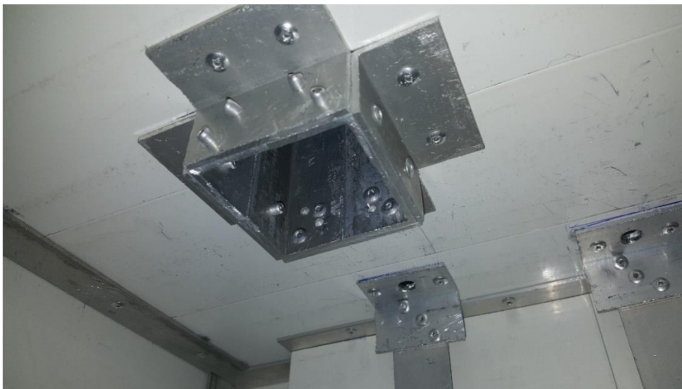
Figure 4.19 Example of using aluminum at a 90 degree angle at the laser descent area from the upper electronics chamber to the heated printing chamber.
