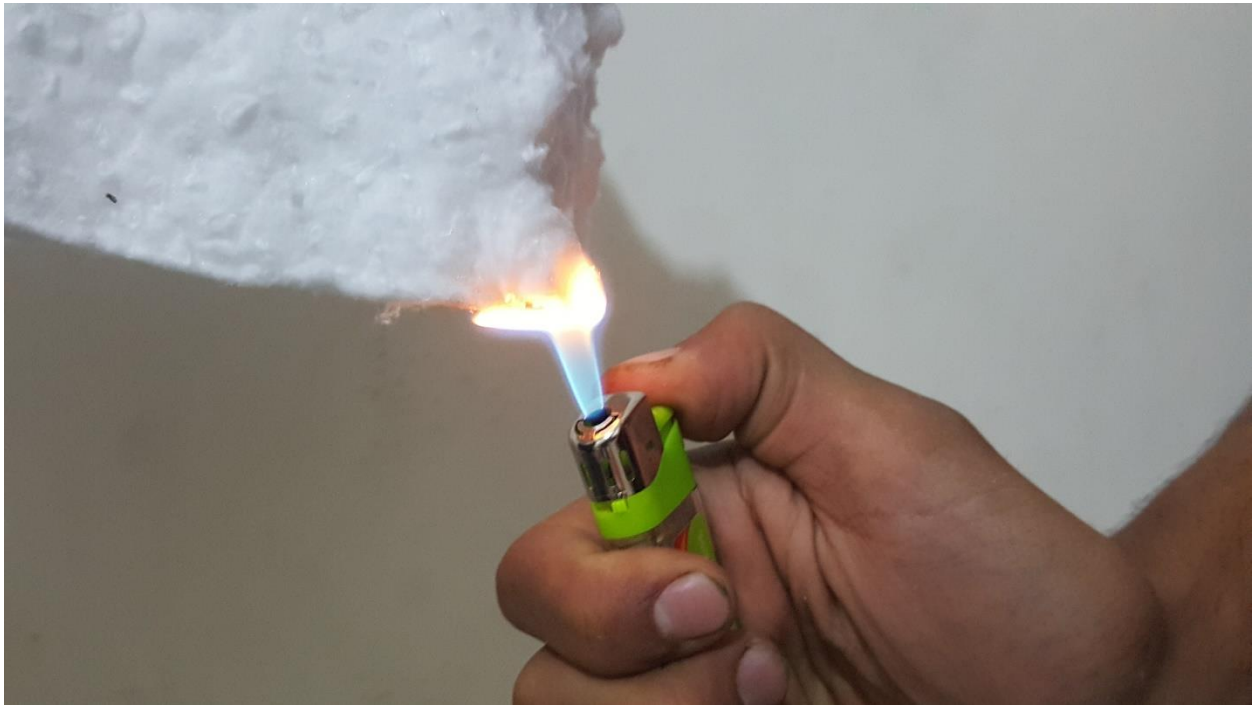
Figure 4.36 Through live experimentation, it is clear how much insulating wool can withstand temperatures, even if they are direct.
