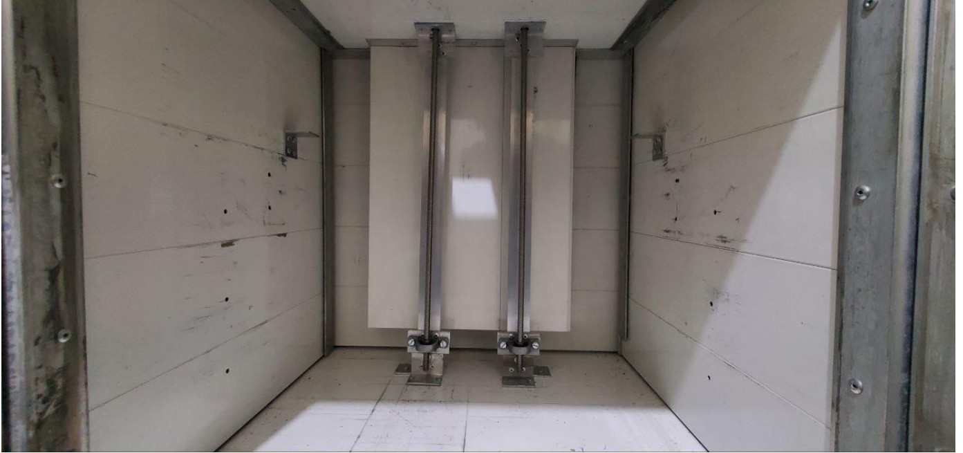
Figure 4.22 Ball screw columns used for transferring the printing room and warehouse, 50cm long and 8mm diameter, responsible for vertical movement up and down.
