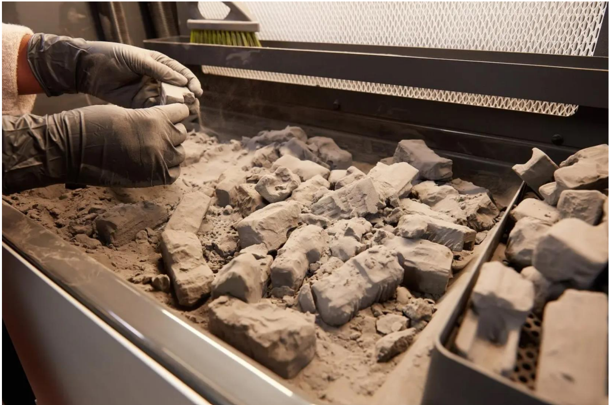
Figure 3.13 Cleaning of finished printed parts buried in powder metal
