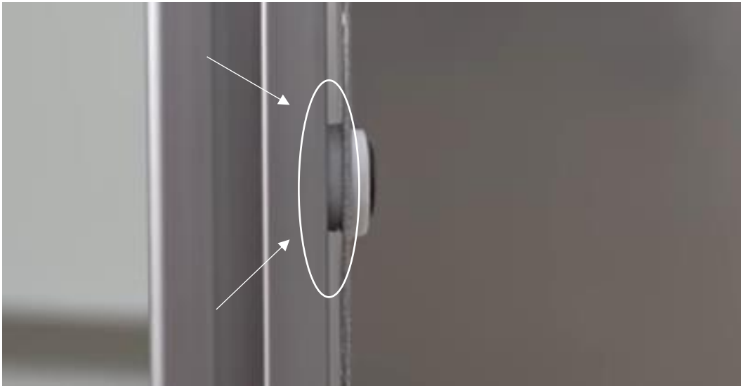
Figure 4.40 Example of where to place the heat-resistant insulating material between the inner and outer walls of the printer.
