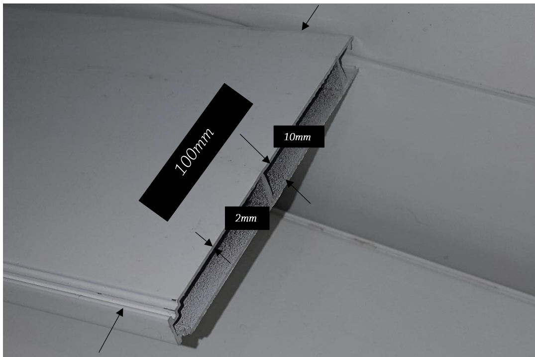
Figure 4.14 Private sector aluminum used in the project instead of aluminum sheets with an explanation of the vacuum gauge and aluminum thickness
