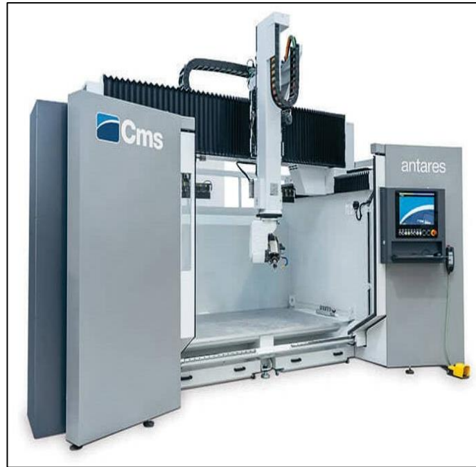
Figure 2.7: 5-Axis high speed CNC machining center with monobloc structure Antares
