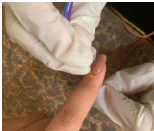
figure(23): Show test and measure the location of the finger in LMRS transmittance mode to 1050nm.
