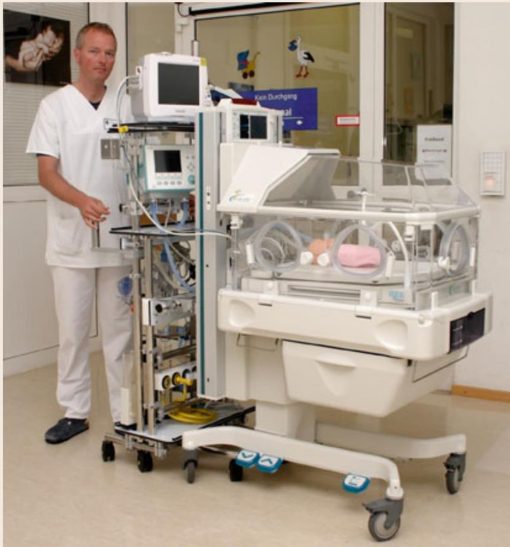
Figure 2-7 Incubator for in-house transportation with docking carriage (courtesy of University Hospital Freiburg and General Electric Company)
