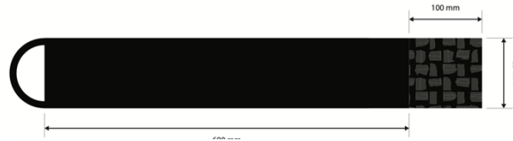
Figure 3.4 Image showing the belt harness for leg support attached to the exoskeleton.
