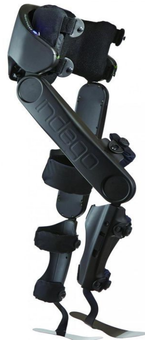
Figure 2.6 : Indego exoskeleton for clinical and personal use
