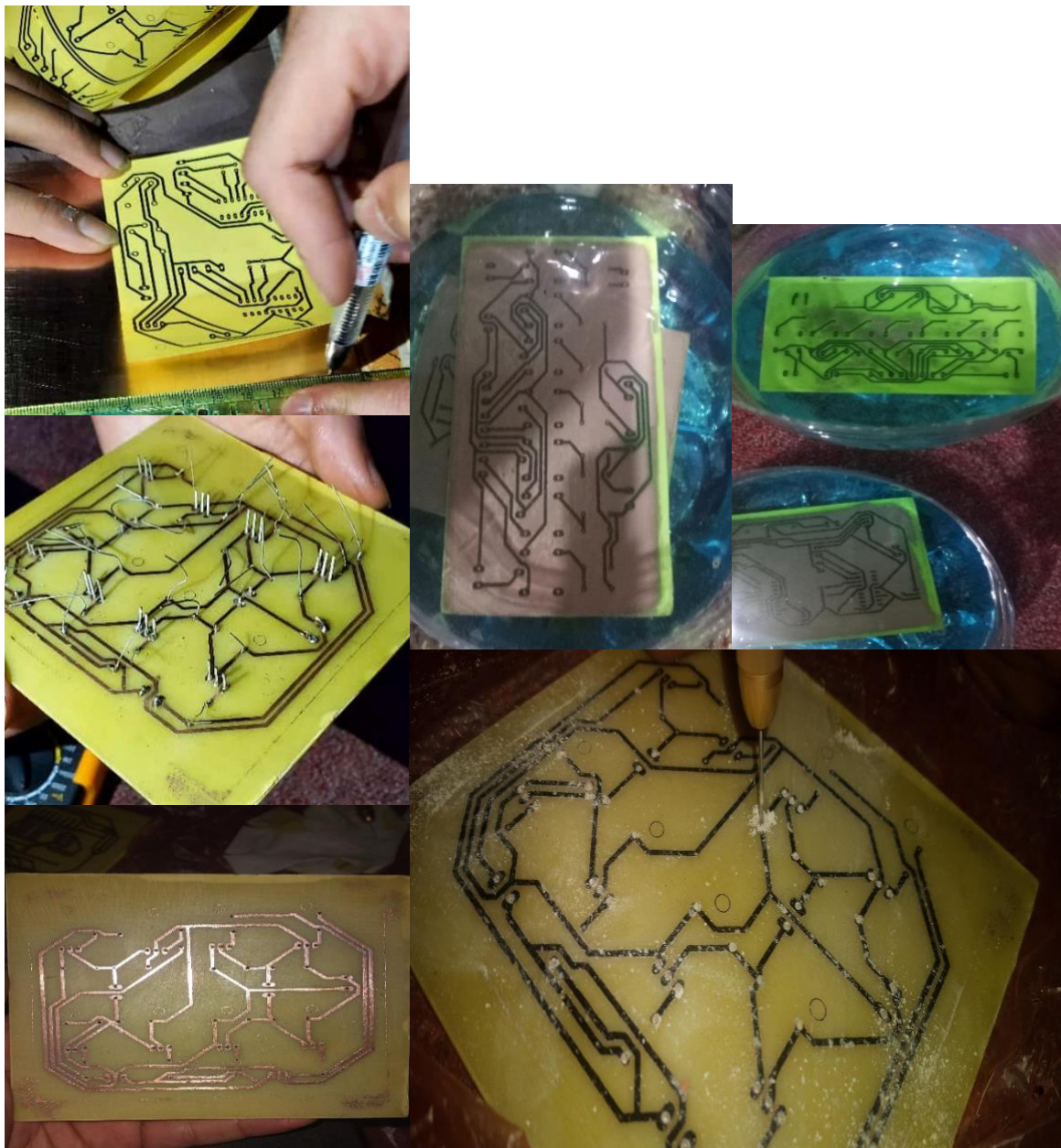
Figure 4.4 : Making a practical board process by hand
