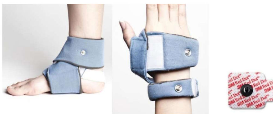
Figure 3.3 Functional straps with incorporated textrodes for TRS measurements(left) and Ag/AgCl 3M traditional electrodes (right)
